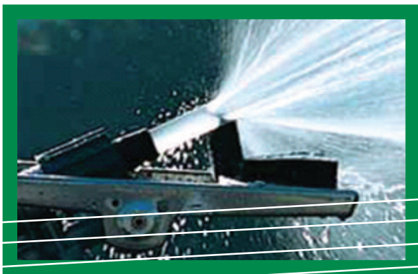
Figure 9.1 Jet-breaker in operation
