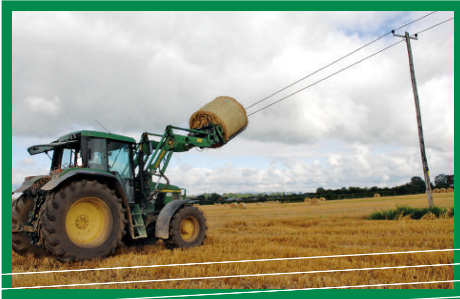
Figure 7.2 Bales on front loader beneath overhead electricity lines
